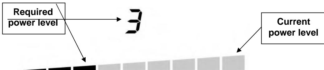
The segments from the power display are turning off one by one until the required power level is reached.
